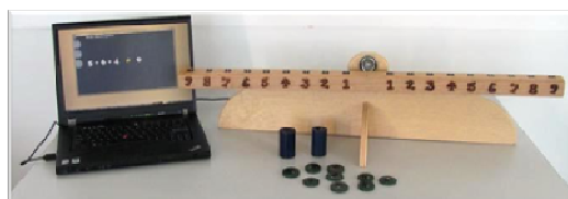
Figure 1. The BEAM. Equations are constructed on a tangible wooden beam with plastic tokens. The graphical user interface is displayed on a tethered laptop.
