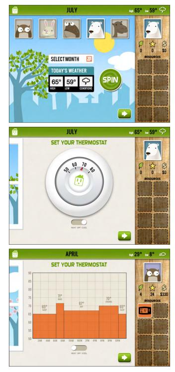
**FIGURE 3.** (top) Your character determines your comfort profile; spin for seasonal weather conditions; (middle) Conventional thermostat interface sets one temperature for the entire day; (bottom) Smart thermostat unlocked with a Resource card lets players set different temperatures for different periods of the day. Artwork by Maisa Morin.
