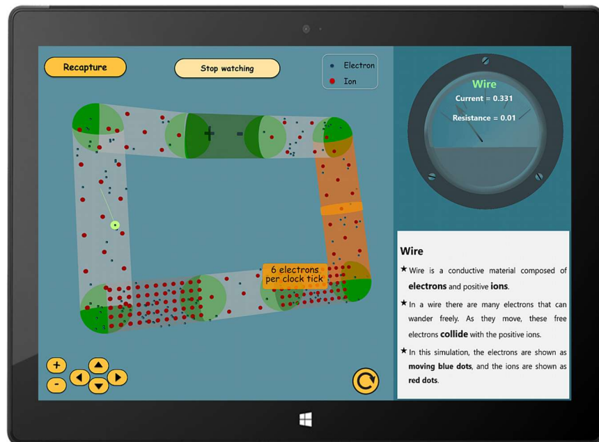
Figure 2. Electron model display. The blue dots are moving electrons and the red dots represent ions in conductive materials. Resistors have higher ion densities than wires.
