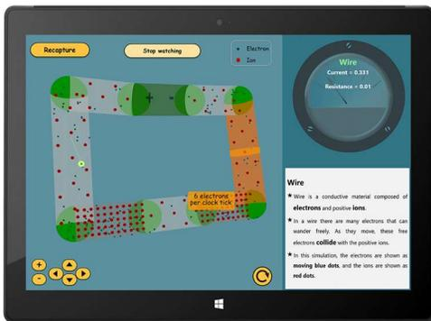
Figure 4. The electron model display in *Spark*. The blue dots are moving electrons and the red dots represent ions in conductive materials. Resistors have higher ion densities than wires.
