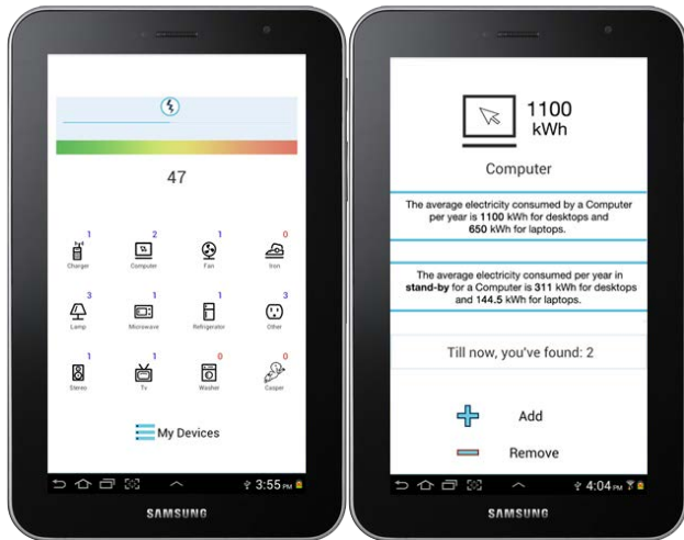
Figure 4. The Ghost Hunter app indicates the strength of an electro-magnetic field (top left) using a combination of visual, auditory, and haptic feedback. The app displays a list of icons (left) showing common devices and appliances. The details screen (right) shows typical consumption levels.
