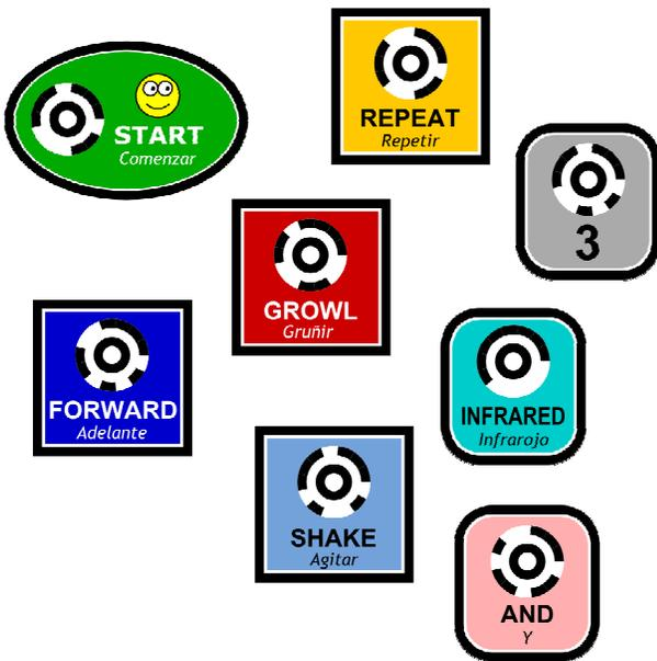
**Figure 4: A selection of faceplates for the tangible programming blocks. The round black-and-white symbol is used by the computer vision algorithm to determine the position, orientation, and type of each block.**
